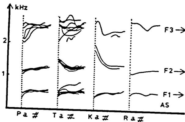
Fig. 3: INVARIANT TARGETS Display of the temporal course of the three first formants, in the vowel /a/, preceded by a labial, dental, velar or uvular consonant and followed by a pause, for the speaker AS. The data have been time-aligned on the vowel onset, found by the automatic segmentation program. The target F-values derived by visual inspection are indicated by arrows on the right part of the figure.
